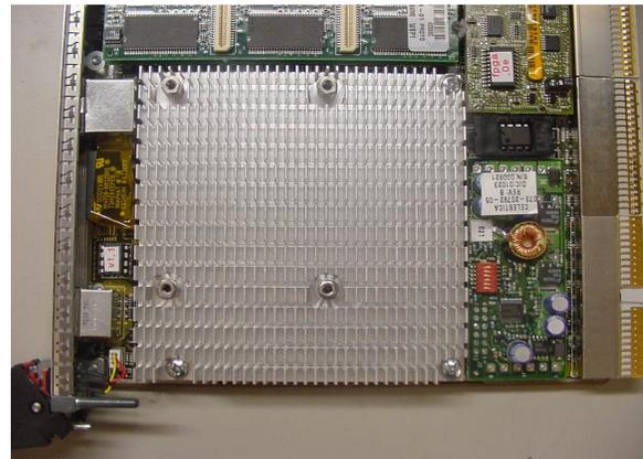
Figure 3. Compact PCI card and heatsink cavity resonances .
