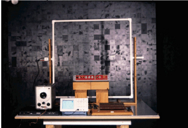
Figure 1. Use PVC pipe to make a loop for magnetic field immunity testing.
